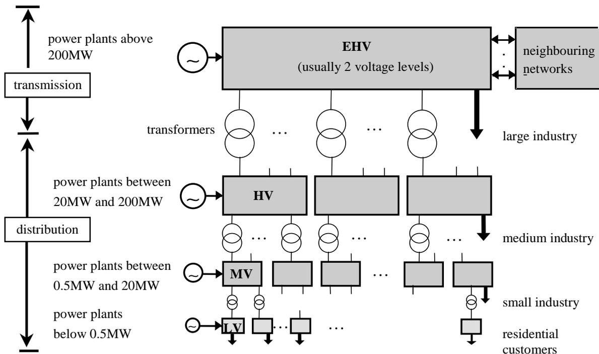
Fig. B.2: Typical network structure in European countries (MW limits for power plants are approximate values)
