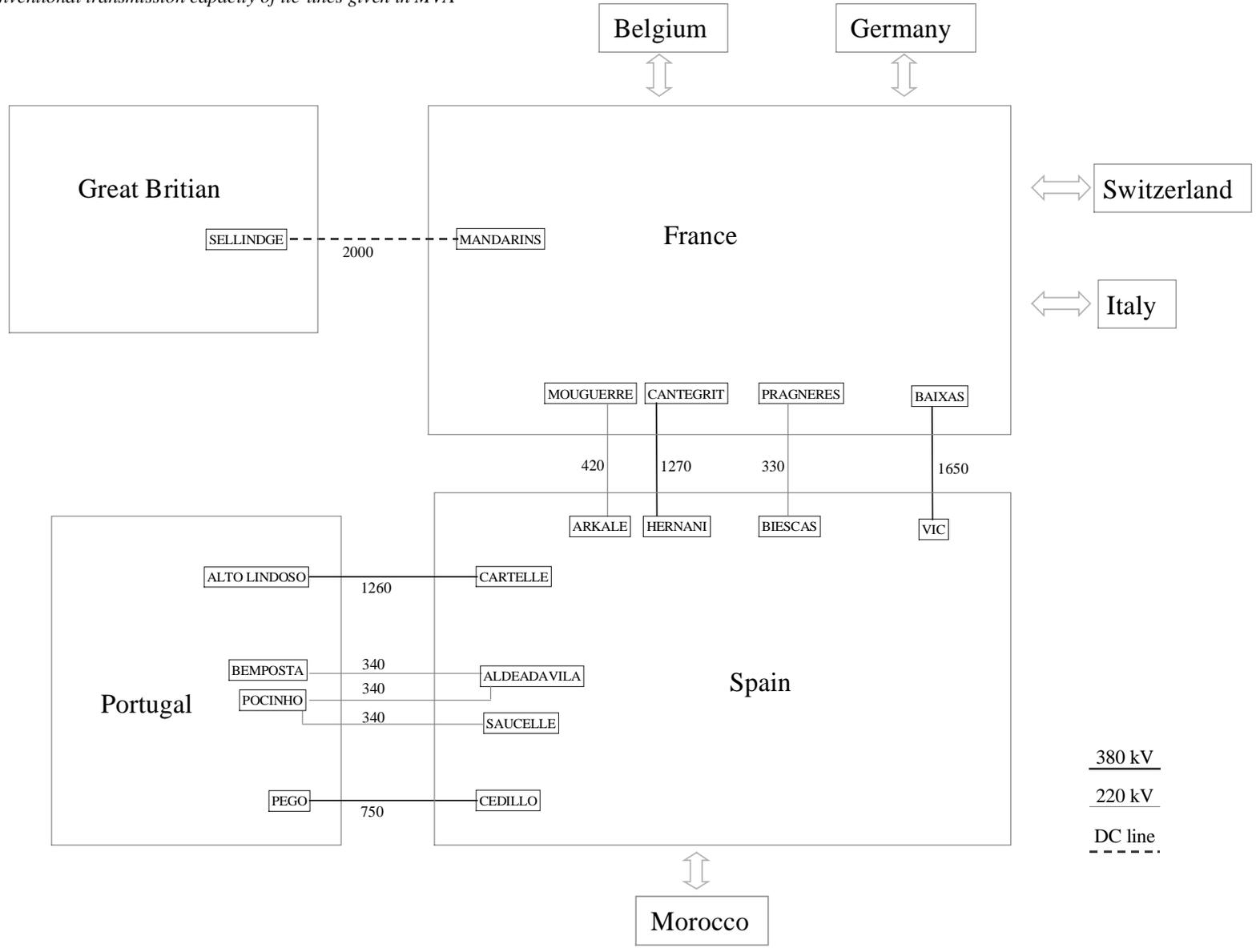
Fig. C.3: Cross-border lines between France, Great Britain, Spain and Portugal (capacity values in MVA, except for DC lines)
