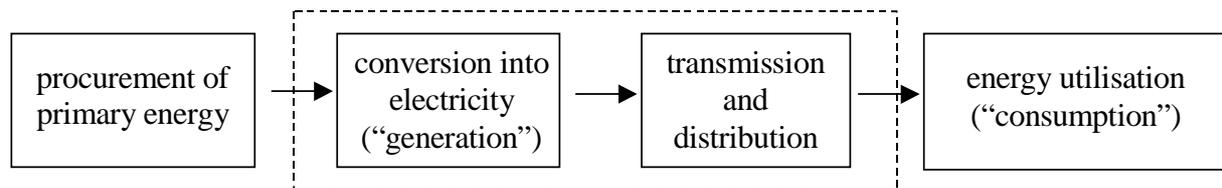
Fig. B.1: Subsystems of electrical power supply
